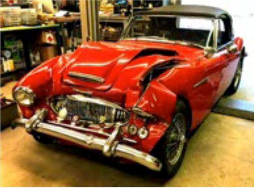
only problem was that one front wheel was skewed outwards because of a bent frame. I decided that it was easier to fix than it was to try and repair the race car.
