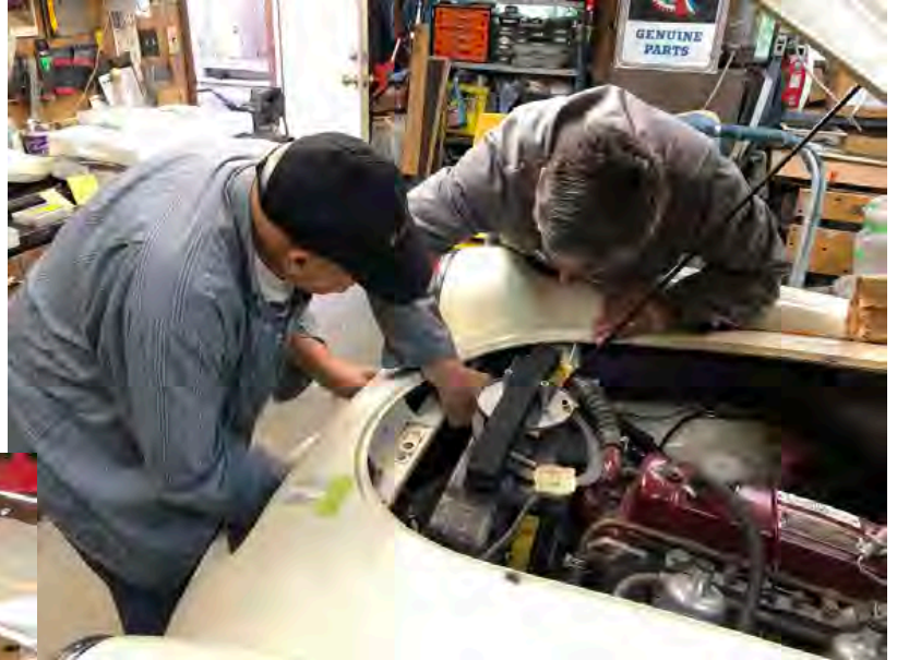
John and Neil fettling the heater vent hose.. much better fit now and we may get some more air out of the heater box.
